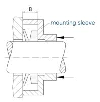
V-ring installation with mounting sleeve
