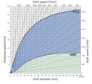
The diagram is for no-pressure operation and favourable conditions with regard to lubrication and heat dissipation (type OS-F10).
